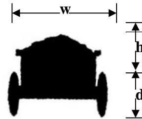
**Dry System-** measure all dimensions in feet and tenths of feet. (1 3/16" is approximately 1/10 of a foot)
